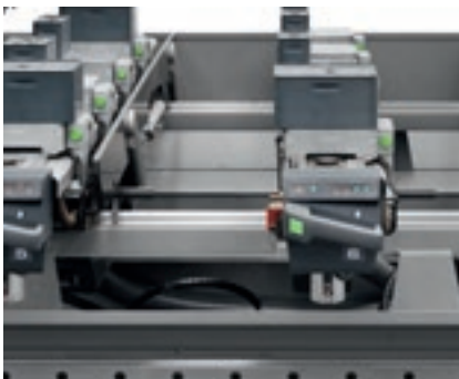
SA (Set Up Assistance) The assisted set-up system, indicates to the operator where to position the panel, pods and rails to avoid potential collisions with the tool.
